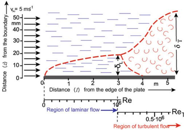
**Fig. 3.63** Formation of laminar and turbulent flow profiles near a planar plate. As an example, the numbers correspond to a flow of air ( $\nu = 1.5 \cdot 10^{-5} \text{ m}^2 \text{ s}^{-1}$ ) with a velocity  $v_\infty = 5 \text{ ms}^{-1}$ . The thickness of the laminar ( $\delta_L$ ) and the turbulent boundary layer ( $\delta_T$ ) are calculated according to the equations in Table 3.2
