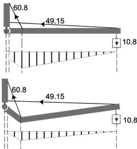
**Fig. 3.58** Two steps for the optimization of the bending load of the forearm. The two muscles which held the forearm bone must generate forces of 60.8 N and 49.15 N, respectively, to compensate the loading force of 10.8 N at its end. These muscle forces are identical in both cases. The bending force of the bone, expressed by the graphs below, however, are quite different. Compare this scheme with the real situation in Fig. 3.57a (Redrawn after Pauwels 1980)
