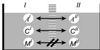
**Fig. 3.17** The derivation of the Donnan equilibrium. Phases I and II are separated from each other by a membrane, that is permeable for the anions (A) and cations (C), but not for the charged molecules M
