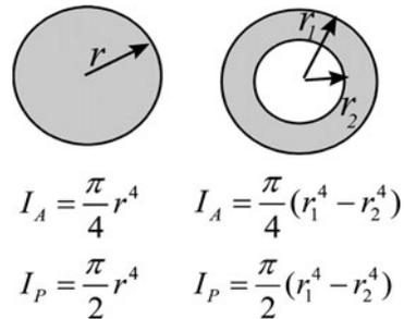
**Fig. 3.60** Area moment of inertia ( $I_A$ ) and polar moment of inertia ( $I_P$ ) for a solid shaft and a tube
