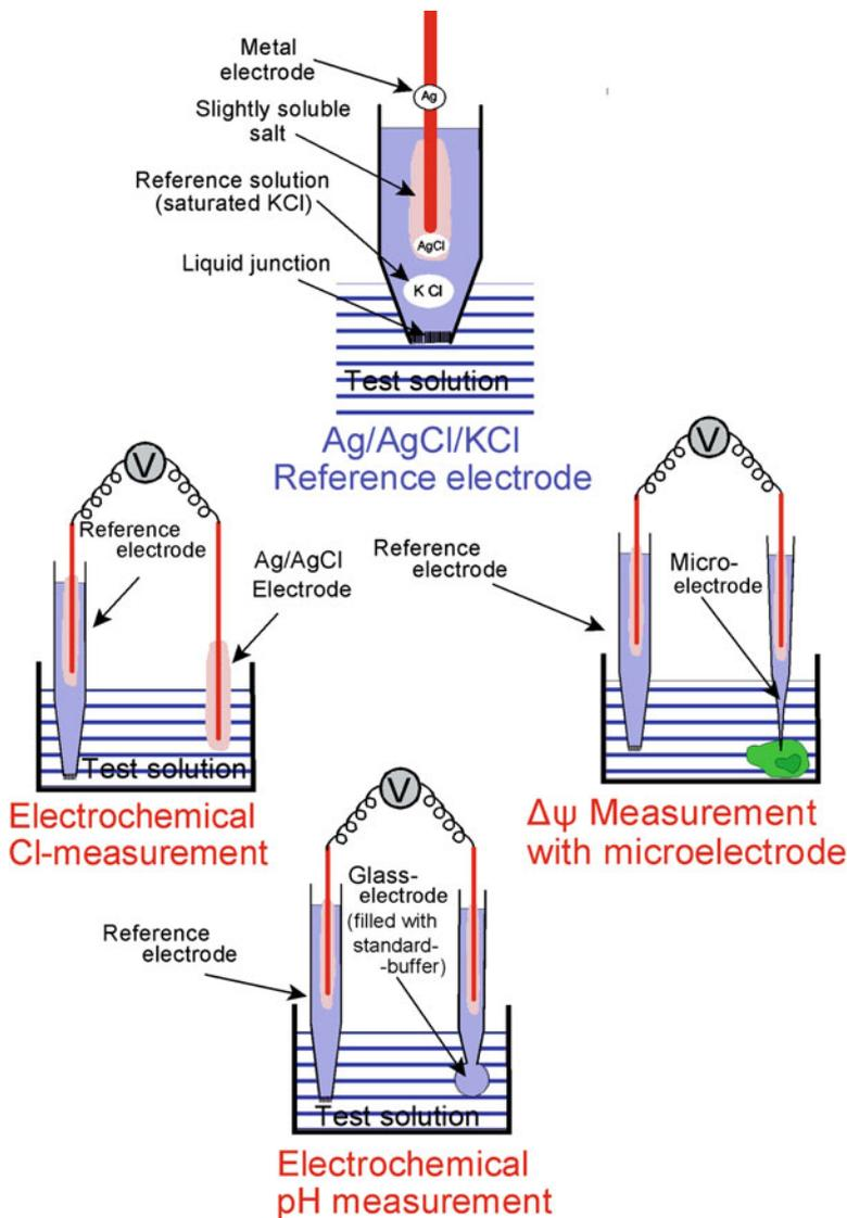
**Fig. 3.16** The construction of an Ag/AgCl/KCl-reference electrode, as well as its application for electrochemical measurements of Cl<sup>-</sup> activity and pH, and as a reference electrode in electrophysiology
