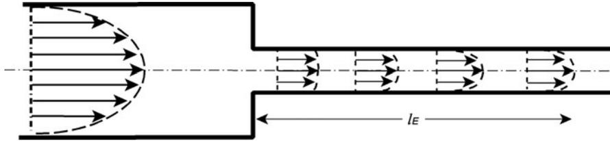
**Fig. 3.66** Laminar flow in a tube: the parabolic velocity profile changes during a sudden narrowing of the tube's radius (entrance effect). Only at a distance  $l_E$  is a new parabolic profile established again
