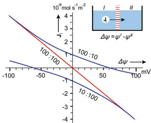
**Fig. 3.23** The flux ( $\mathbf{J}_i$ ) of a univalent cation ( $z_i = +1$ ,  $P_i = 10^{-7} \text{ ms}^{-1}$ ) driven by a concentration, as well as an electrical potential gradient according to the Goldman equation (3.160). The concentrations in phases I and II are listed on the curves. Description in the text
