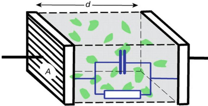
**Fig. 3.39** A capacitor consisting of two parallel plates of area  $A$ , and a mutual distance  $d$ , filled with an inhomogeneous medium (e.g., cell suspension or biological tissue). Neglecting the real dielectric heterogeneity, it can be described formally by a RC-circuit (blue)
