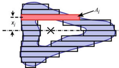
**Fig. 3.62** Determination of the second moment of area of a tubular bone by a graphical method. The profile of the bone is approximated by many rectangles with individual areas  $A_i$  and distances from the neutral plane (---)  $x_i$ ; X – center of gravity
