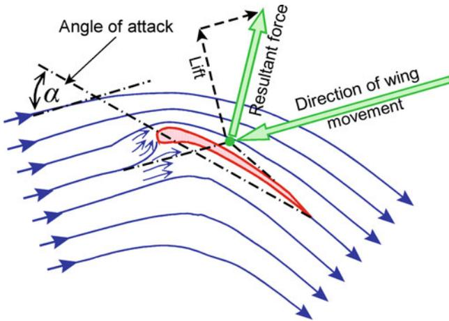
**Fig. 3.72** Air stream and forces of bird flight during a stroke of the wing forwards and downwards (Redrawn after Hertel 1963)
