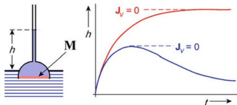
**Fig. 3.22** The height of the water column in a Pfeffer osmometer dependent on time in two experiments under different conditions: Pfeffer's cell is closed by a semipermeable membrane (**M**) (red line), and: solvent as well as solute can penetrate the membrane (blue line). The conditions with stationary pressure in this manometer ( $dh/dt = 0$ , i.e.,  $dp/dt = 0$ ) mean at the same time stationary volume ( $dV/dt = \mathbf{J}_V = 0$ )
