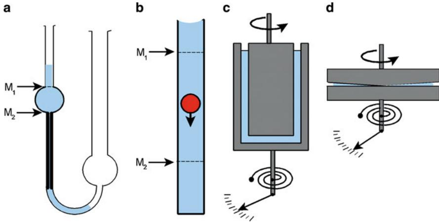
**Fig. 3.53** Various setups to measure the viscosity of fluids. (a) Capillary viscosimeter after Ostwald, (b) viscosimeter with falling sphere, (c) coaxial-type rotational viscosimeter, (d) cone-type rotational viscosimeter
