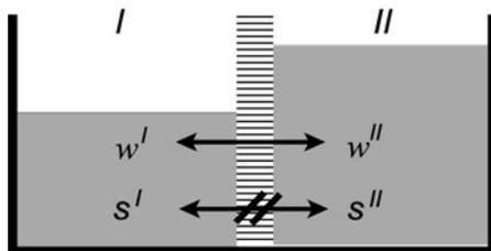
**Fig. 3.11** Derivation of osmotic pressure: Phases I and II are separated from each other by a semipermeable membrane. Only the solvent ( $w$ ), but not the solute ( $s$ ), can penetrate this membrane. The hydrostatic pressure of both sides of the membrane is different
